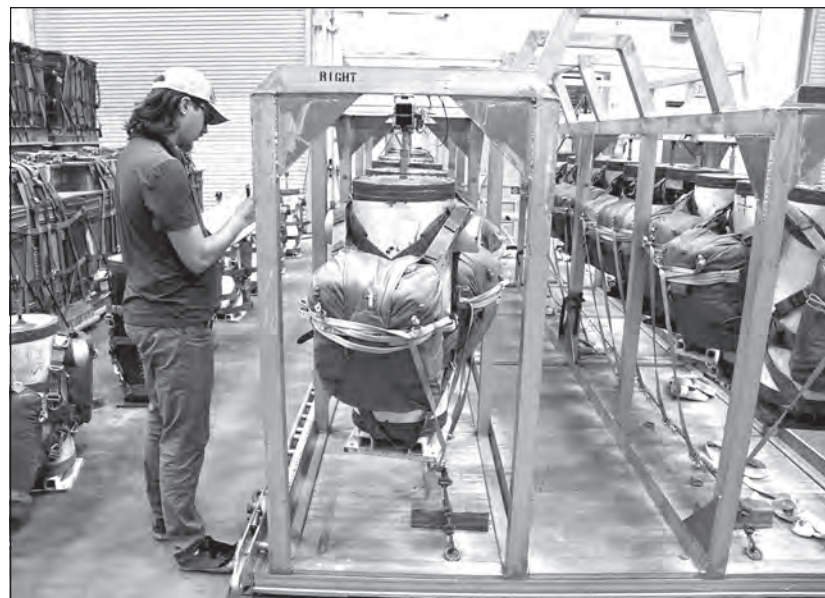
The T-11 personnel parachute offers jumpers a slow and stable descent, especially in high winds, and can support more weight than previous parachutes, a crucial advantage for warfighters who carry robust, heavy gear. Now long-fielded, the T-11 is still returning to Yuma Proving Ground for further refinements and improvements, including recently evaluated modifications to the corner vents. (Photo by Mark Schauer)
