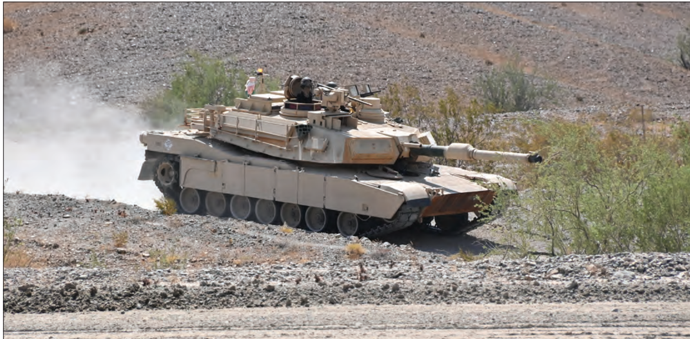
U.S. Army Yuma Proving Ground testing has touched virtually every aspect of the M1 main battle tank. The most recent example is a test to verify new fire control software meant to improve the speed and accuracy of the platform's 120mm gun, .50 caliber and 7.62 machine guns, and grenade launchers, all while ensuring other aspects of the vehicle's performance are not degraded. (Photo by Mark Schauer)
