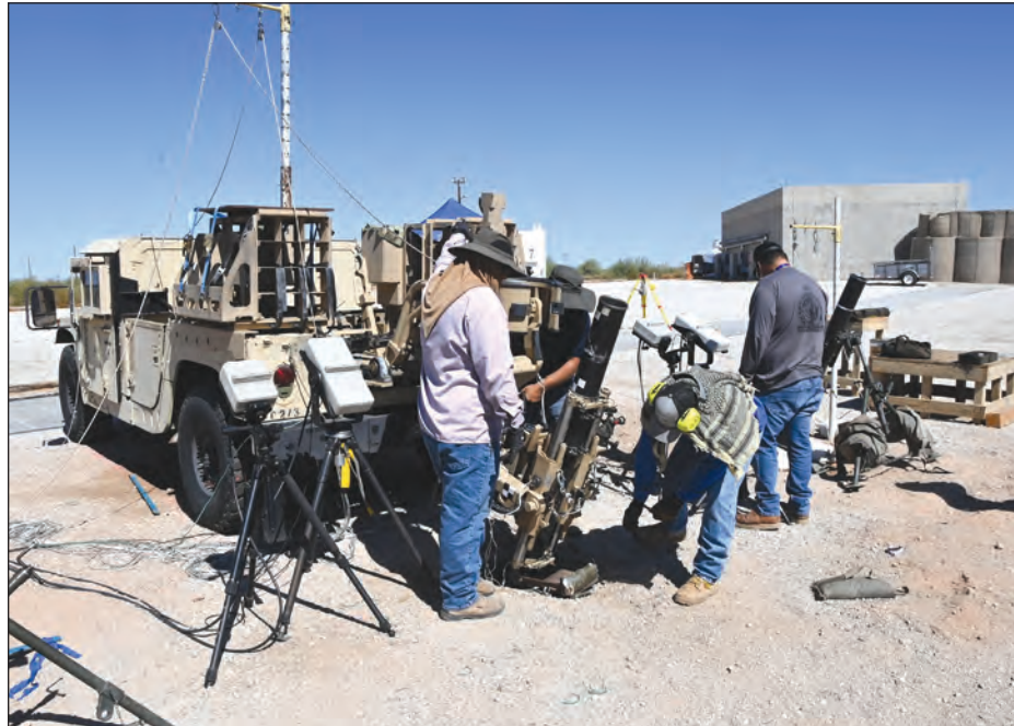
U.S. Army Yuma Proving Ground (YPG) recently conducted a characterization test of the Sling mobile mortar system. The mortar is a standard 120 mm tube with the sling system and fire control system mounted to the back of a military vehicle. The weapon can be automatically deployed and emplaced in less than one minute and fire up to 16 rounds in the first minute of fire, four rounds per minute for extended periods of time thereafter. (Photo by Mark Schauer)
