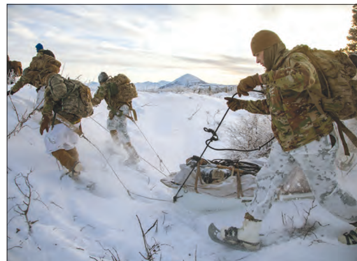
LEFT: On a typical day, Soldiers would pack the Arctic Mobility Sustainment System sled under test with the tent, a heater, and their basic standard issue items for Arctic infantry operations, then pull the sleds in either nine-Soldier squads or four to five Soldier teams as U.S. Army Cold Regions Test Center’s test personnel led the way. RIGHT: Moving the heavy sleds across U.S. Army Cold Regions Test Center’s hilly tundra and thickly forested areas is challenging in any condition, but particularly so in the extreme cold and deep snow of winter. (Photos by Sebastian Saarloos)
