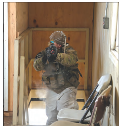
Even when outfitted with a flash suppressor, the XM7 weighs less than 10 pounds. The new weapon has a standard rifle scope with an etched reticle and adjustable modes of operation where it can act like a red dot or close combat optic.
