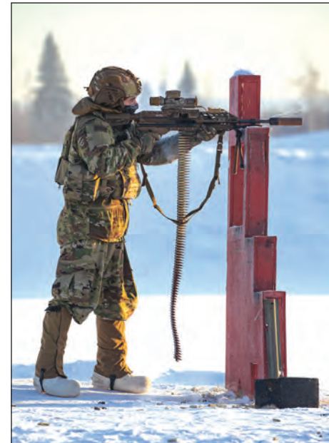
The U.S. Army Cold Regions Test Center staged a multiweek test of the Army's Next Generation Squad Weapon early this year. The XM7 and XM250 are successors to the M4 rifle and M249 light machine gun that American forces have used for decades. The new weapons boast improved accuracy and range, weigh less, and fire with less recoil, even though its 6.8-millimeter (mm) round is larger than the two legacy weapons' 5.56-mm cartridge. (Photos by Sebastian Saarloos)
