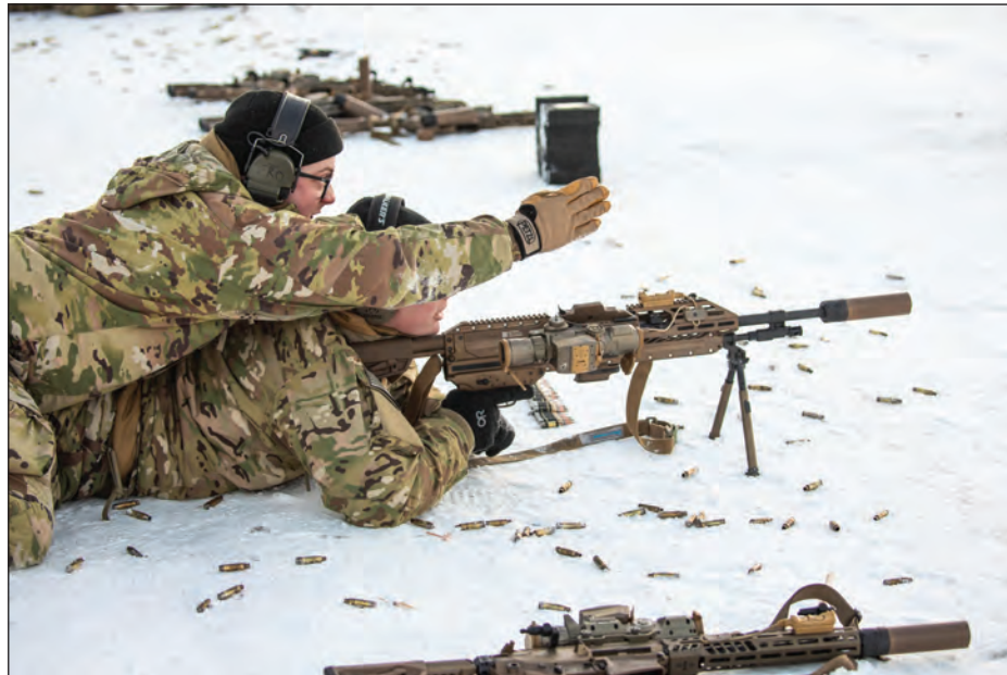
The U.S. Army Cold Regions Test Center staged a multiweek test of the Army's Next Generation Squad Weapon early this year. The XM7 and XM250 are successors to the M4 rifle and M249 light machine gun that American forces have used for decades. The new weapons boast improved accuracy and range, weigh less, and fire with less recoil, even though its 6.8-millimeter (mm) round is larger than the two legacy weapons' 5.56-mm cartridge. (Photos by Sebastian Saarloos)
