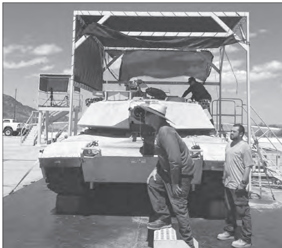
Charles Lott, of the System Test Branch, (center) performs a bore sighting of the gun barrel of an M1-A1 Abrams tank prior to a firing test. Also pictured are Direct Fire Team Lead Hector Vergara (top right) who is speaking to the driver of the tank while a coworker (bottom right) looks on. (Loaned photo)
