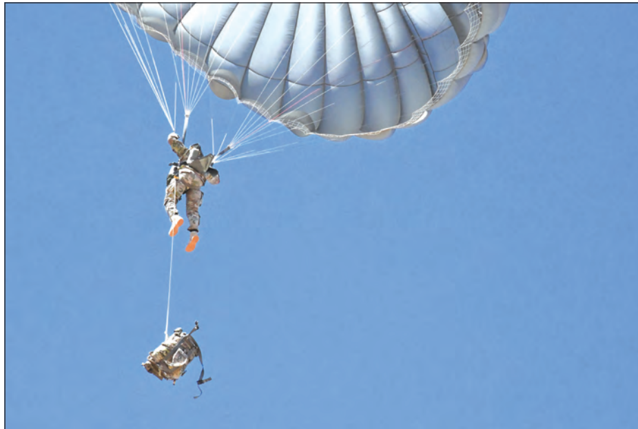
The U.S. Army Airborne Test Force at Yuma Test Center recently conducted parachute jumps to test the survivability of Manpack radios inside the Army's newest Radio Carrier Rucksack. When jumpers were about 150 feet from the ground, they lowered the rucksack carrying the radio, making it about 15 feet below them when they landed. (Photo by Ana Henderson)
