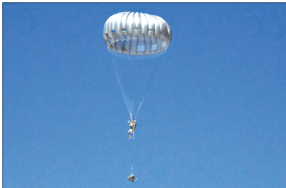
The harness single point release is the equipment that secures the ruck close to the jumper’s body and is designed to be lowered on a release line away from the jumper just prior to landing. When the Soldiers were about 150 feet from the ground, they lowered the rucksack carrying the radio, making it about 15 feet below them when they landed. (Photos by Ana Henderson)
