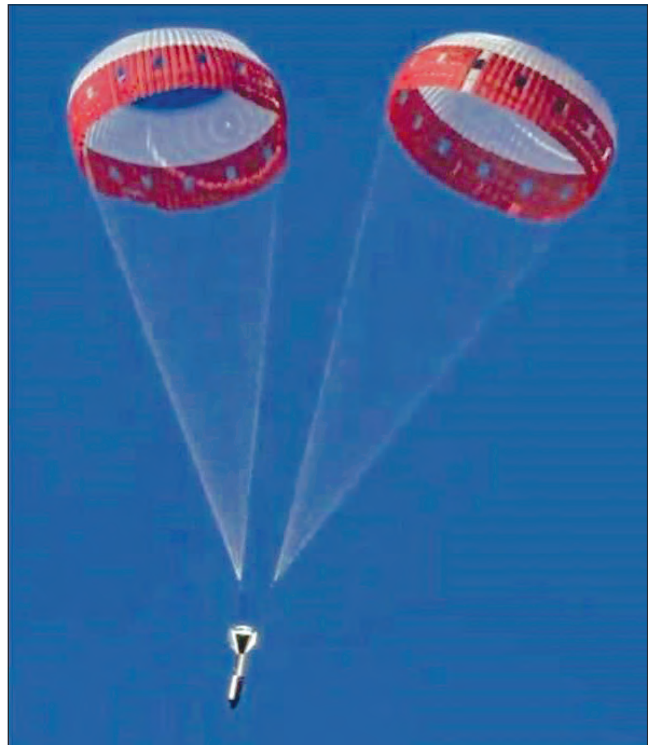
After a small modification to the Boeing Starliner’s main parachute’s soft links, which connect the suspension lines to the riser extensions, engineers set out to prove the system in a real-world test on a remote drop zone at YPG. (Photo courtesy of Steven Siceloff)
