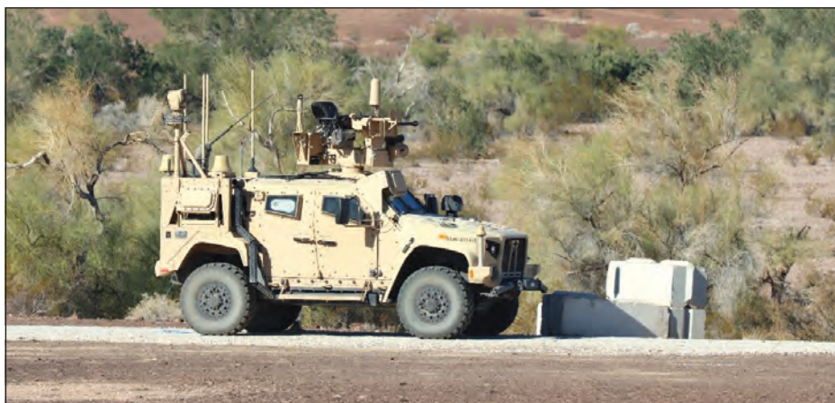
U.S. Marines with Marine Corps Systems Command, fire a Stinger Missile from a Marine Air Defense Integrated System (MADIS) at Yuma Proving Ground, Dec. 13, 2023. The MADIS Mk1 and Mk2, pictured, form a complementary pair and will be the basic building block of the Low Altitude Air Defense Battalions' ground-based air defense capability. (Photo by Virginia Guffey)
