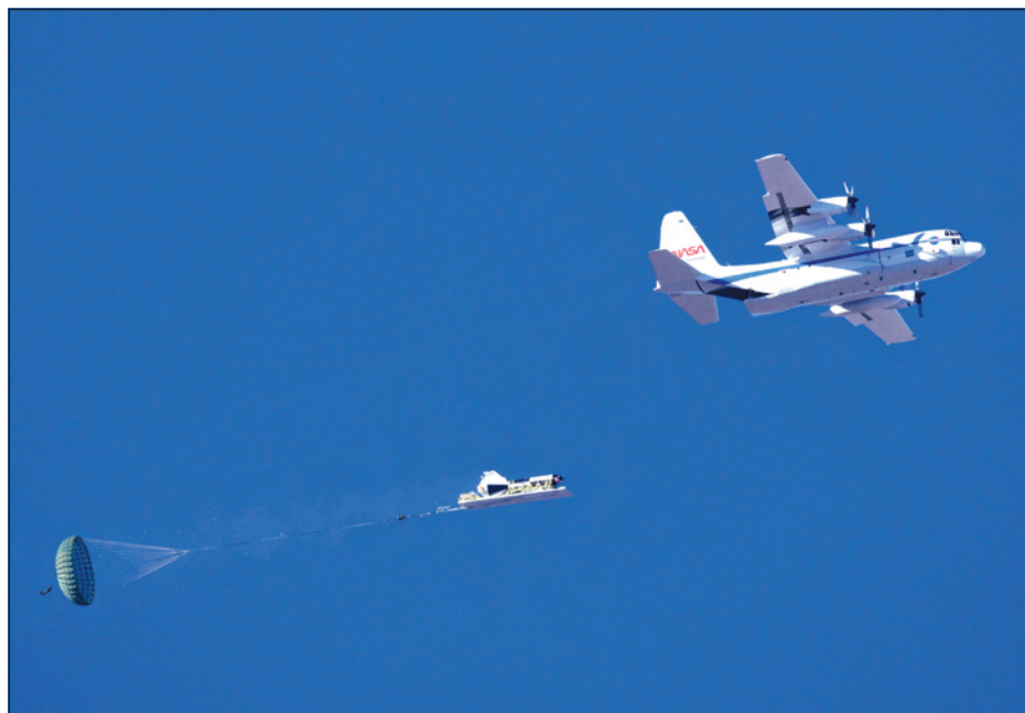
A NASA test of the Boeing Starliner’s main parachute system took place at U.S. Army Yuma Proving Ground (YPG) on Jan. 9, 2024. The test dart was dropped from a NASA C-130 cargo plane flying at an altitude of 13,000 feet at 145 knots air speed. (Photo by James Blair)
