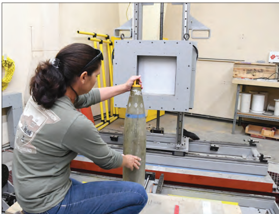
Radiography Technician Lindsey Carter holds a 155-round on the TXR panel for digital radiography. The machine can perform a nose and base x-ray. The team usually takes a 0- and 90-degree x-ray of each round. (Photo by Ana Henderson)
