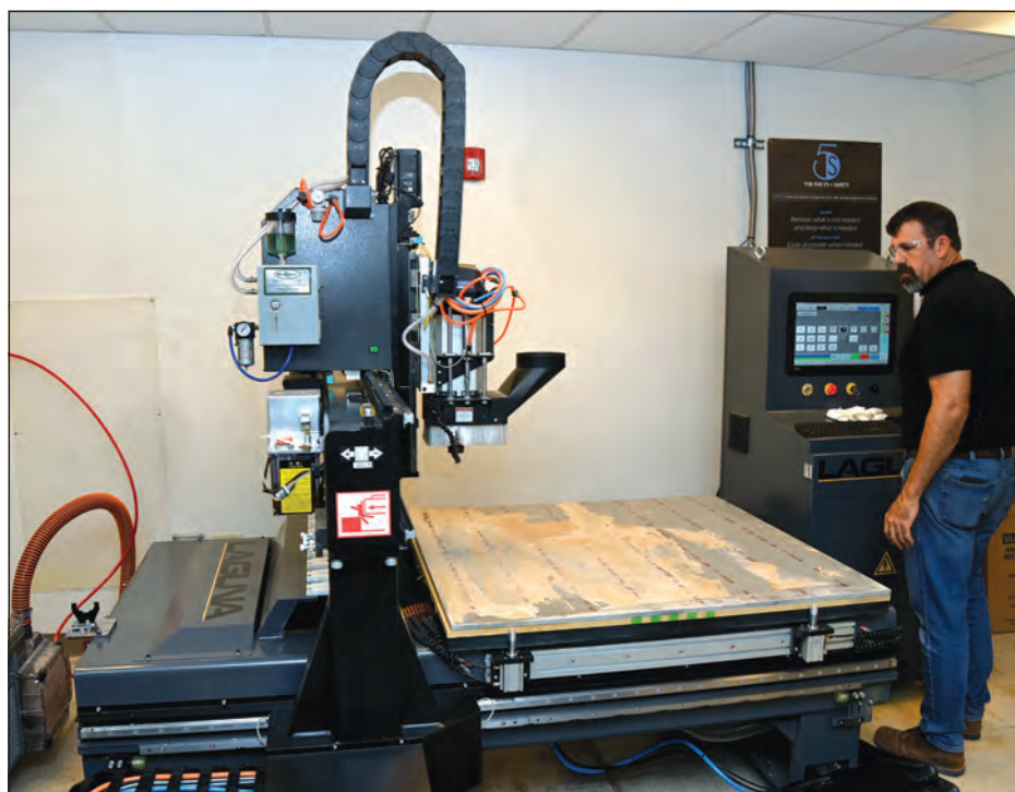
Electro Optical Maintenance (EOM) Lab Supervisor Drew Trujillo uses the lab's recently-acquired router table. The EOM lab is responsible for the maintenance, repair, and even design of a variety of equipment, from cameras and lenses to bomb-defusing robots. It also designs and fabricates custom items to support the testing work force. (Photo by Mark Schauer)
