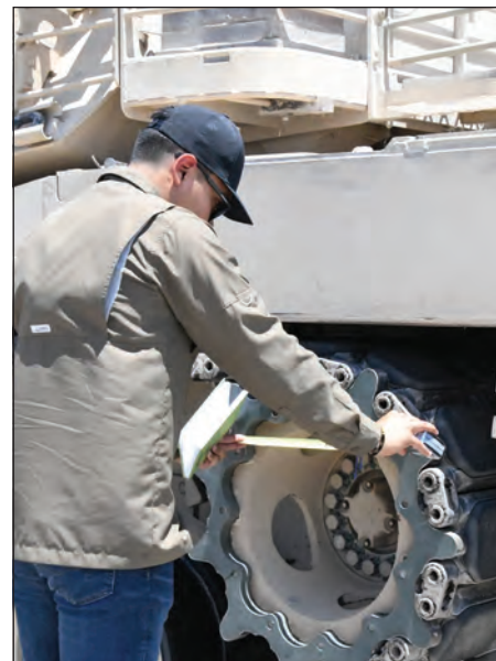
Combat and Automotive Systems Division intern Richard Santiago performs an inspection on the track and sprocket of an Abrams M1A2 SEPv3.
