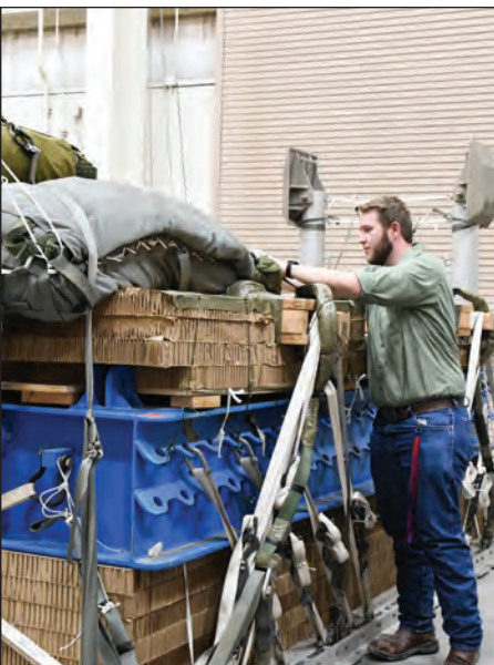
Air Delivery intern Jay Clark checks tags on a tub, verifying the weight which simulates the weight of a test vehicle and that the parachutes are connected. (Photos by Ana Henderson)
