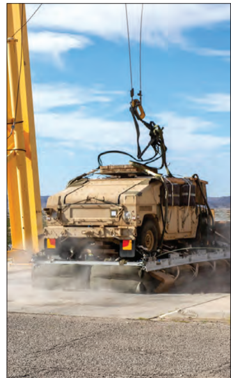
Conventional cargo payloads are typically cushioned with a honeycomb-like cardboard material. RRDAS, dramatically reduces the amount of honeycomb necessary to dissipate the force of impact with 10 reusable airbag modules. The self-inflating airbags can be utilized as low as 750 feet above ground level and carry loads from between 5,000 and 22,000 pounds.
