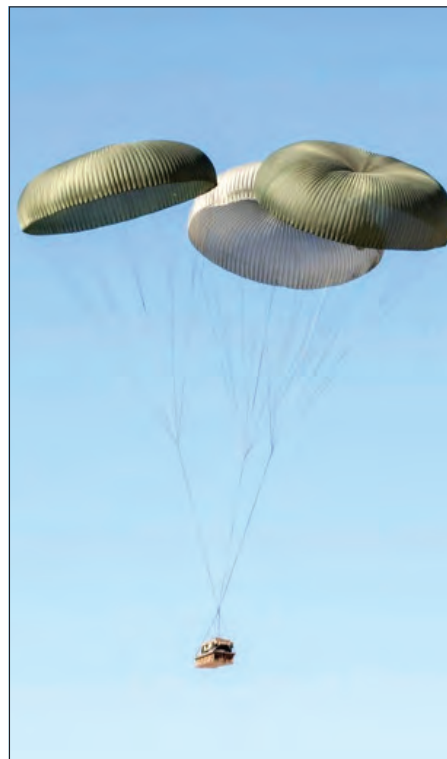
U.S. Army Yuma Proving Ground has been testing the Rapid Rigging De-Rigging Airdrop System which promises to get Soldiers out of a drop zone and into the fight with the equipment they need faster than ever. The reduced use of honeycomb should lower rigging time by 25%, but testers are particularly excited about reducing de-rigging time by 40%, which gets Soldiers out of harm’s way faster. (U.S. Army photos)
