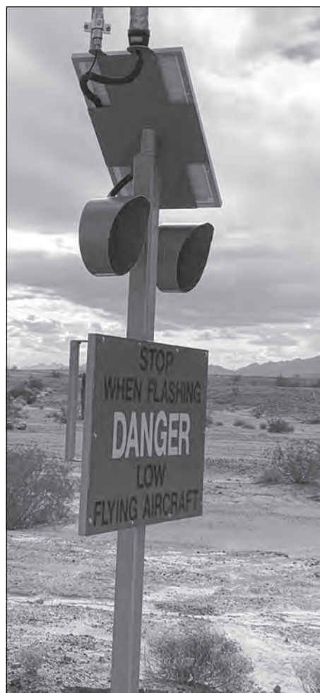
Laguna Airfield air traffic controllers operate the signs located at the intersection of Barranca and Campo Avion Road. They activate the flashing red lights when an aircraft is approaching. Drivers need to stop when they see the flashing lights. When the aircraft has landed, and the lights stop flashing, they can proceed. (Photo by Ana Henderson)
