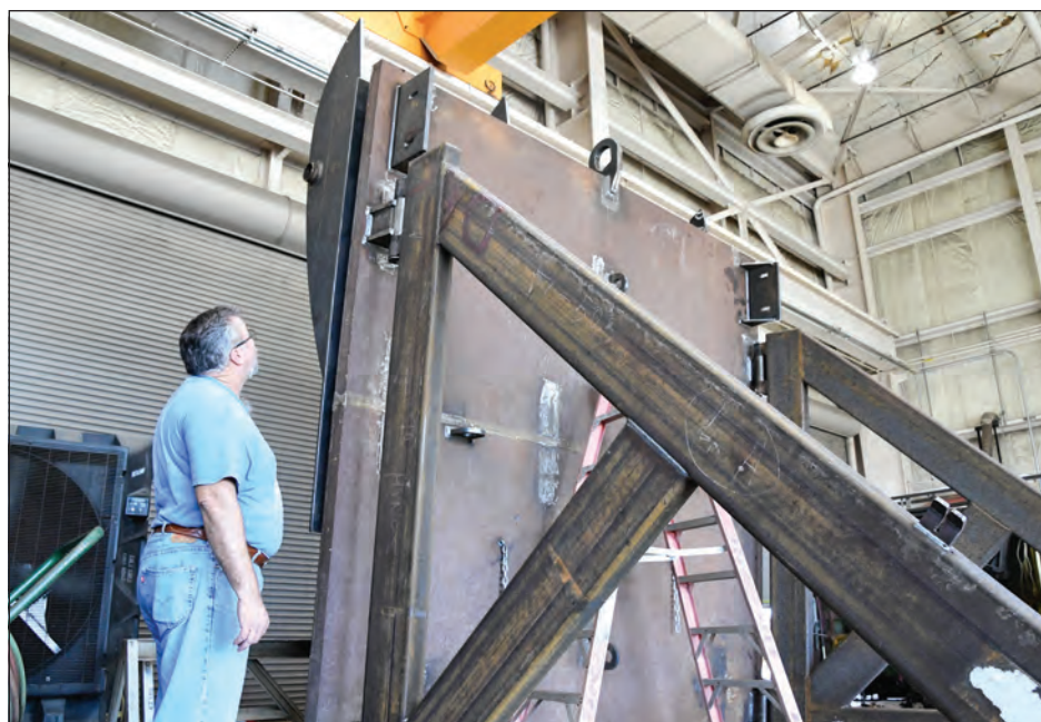
James Ingram the lead engineering tech at Yuma Test Center's Machine Shop stands next to a large mobile blast shield his team fabricated. (Photos by Ana Henderson)
