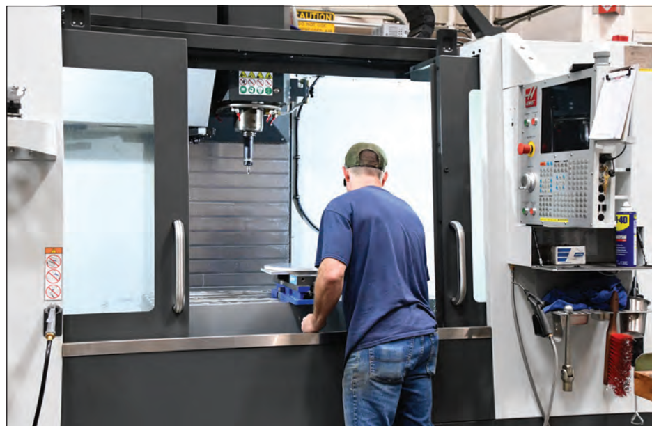
Machinist Matt Keddy is working using a computer numerical control (CNC) machine. The enclosed CNC machines are computer operated — a program must be inputted to instruct the machine what to do.
