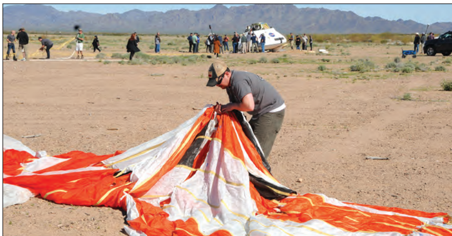
NASA subjected the parachute system of the Orion space capsule to multiple developmental and qualification tests at U.S. Army Yuma Proving Ground (YPG) in recent years. The rope that makes up the parachutes' cord is made of Kevlar, the strong synthetic fiber used in body armor: the change was made from steel because of testing at the proving ground. (Photo by Mark Schauer)
