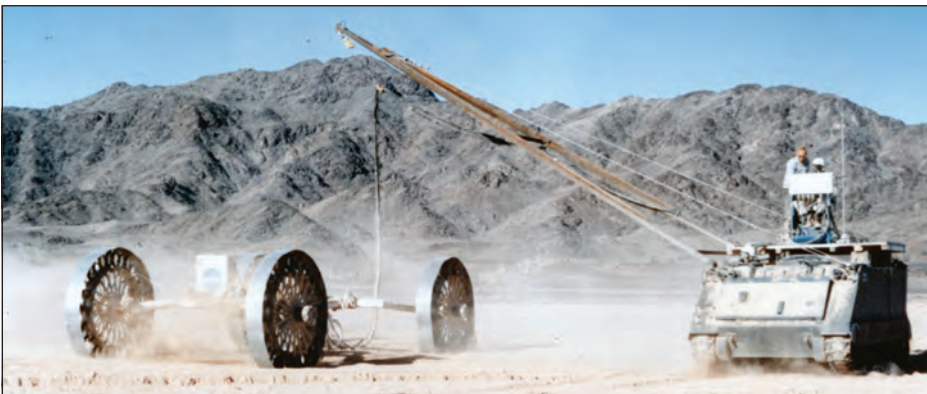
In 1966, the Mobility Test Article, an early version of the lunar rover, went through developmental testing on Yuma Proving Ground's vast ranges. The final product traversed the moon in 1971 and 1972. (U.S. Army photos)
