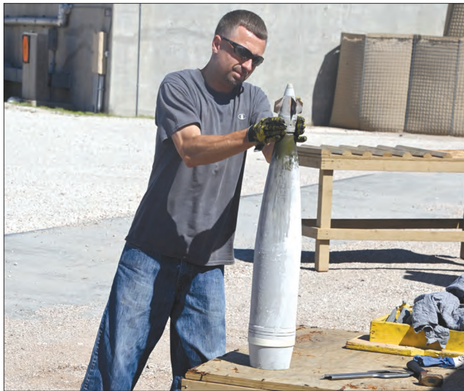
One of the first technologies born of the push for more accurate artillery in the past 20 years was the Precision Guidance Kit (PGK), a screw-on fuze that transforms a conventional artillery round into a guided near precision projectile accurate to approximately 150 feet of a target. U.S. Army Yuma Proving Ground tested PGK extensively throughout its development and continues to do so today. (Photo by Mark Schauer)
