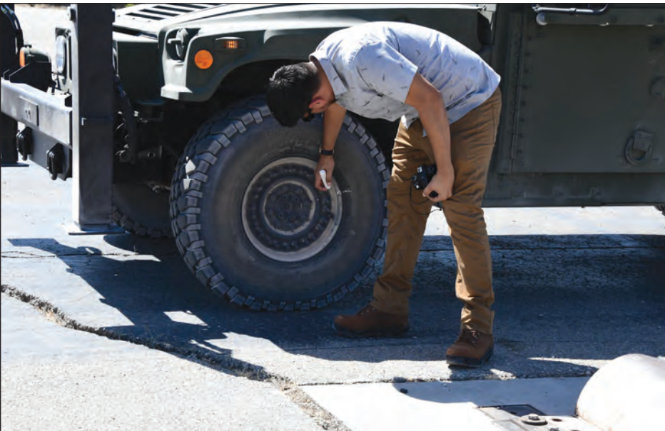
Test Officer Oliver Ramos uses white chalk to mark the tire and wheels to see if there was any slipping “When you apply force sometimes you get slips from the wheel on the tire. So, I mark it to verify that it didn’t move when the full weight is applied,” explained Ramos.
