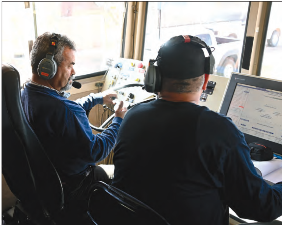
The modern digital controls recently upgraded on the dynamometer improve the precise control of the vehicle's speed and loads applied to vehicles during evaluations, which means more accurate test data for customers. (Photo by Mark Schauer)
