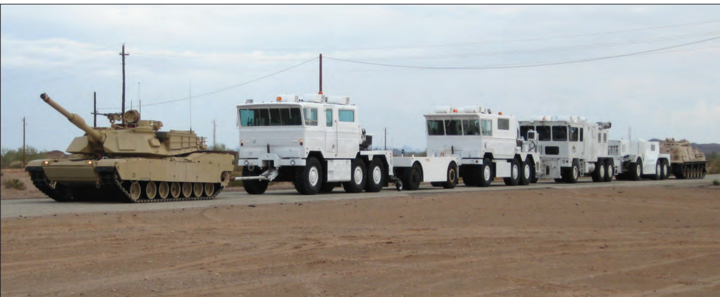
“All vehicles that go through testing at YPG—tracked and wheeled—need to be stressed,” said Jose Rodriguez, electronics team lead in YPG’s Engineering Support Branch. “You want to stress the internals like the transmission and the engine to their breaking limit, and the way to do so is to put them under a load.” (U.S. Army photo)
