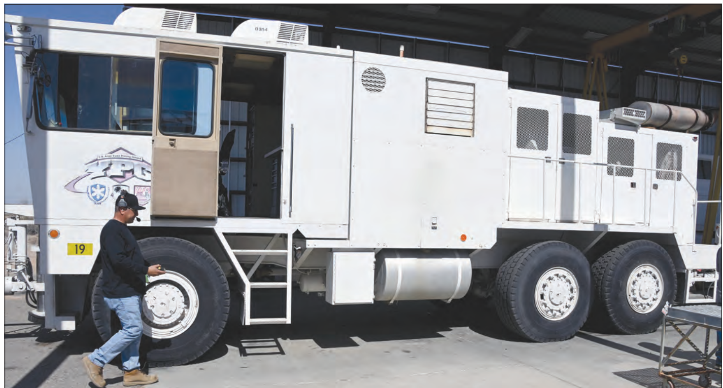
YPG has three massive mobile dynamometers all which were manufactured with analog controls. Recently, YPG fully digitized the newest of the three dynamometers. The modern digital controls improve the precise control of the vehicle’s speed and loads applied to vehicles during evaluations, which means more accurate test data for customers. (Photo by Mark Schauer)
