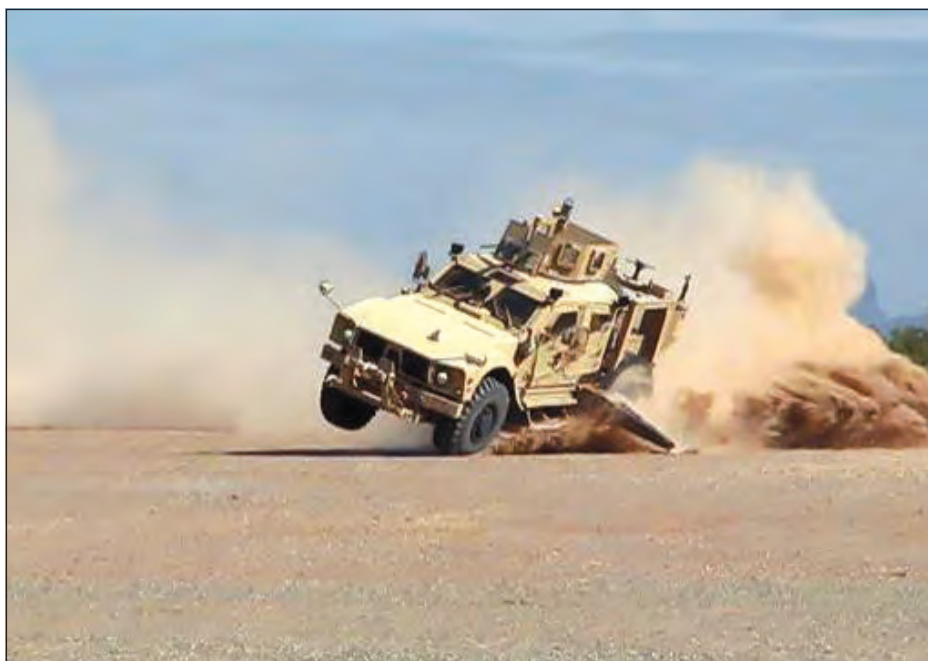
At Yuma Proving Ground (YPG), the Automotive Instrumentation Section within the Instrumentation Division is equipped to test self-driven and driver-aided vehicles. The Mine Resistant Ambush Protected vehicle pictured, is driving at high speeds and teetering side to side as the robot controls the wheel to test for rollovers. (YPG photo)
