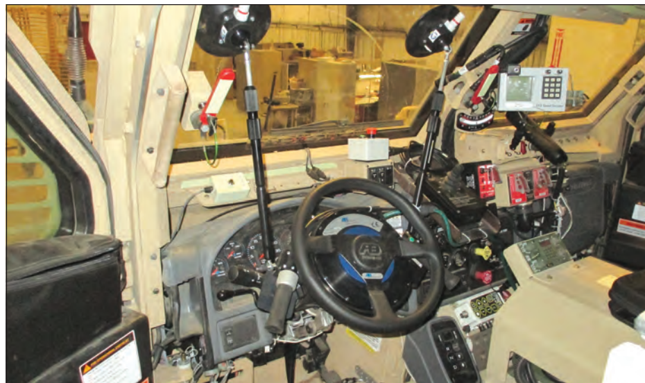
YPG recently acquired driverless robot systems which will be used to test Advanced Driver-Assistance Systems that assist drivers by detecting nearby obstacles or driver errors by responding accordingly, and Automated Driving Systems that perform the driving. The robot is made up of various pieces that attach to the steering wheel, accelerator, and brake pedals. (YPG photo)
