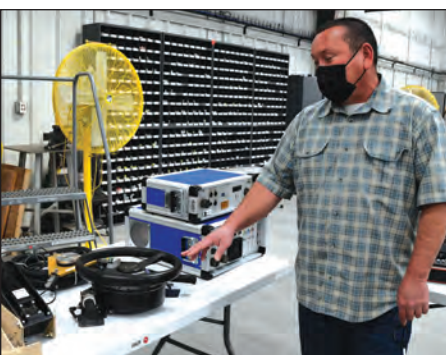
Automotive Instrumentation has used another robot for several years now. It requires a human to be inside the vehicle under test, but the robot takes over when commanded and it’s for more extreme maneuvers to test Electronic Stability Control. (Photo by Ana Henderson)
