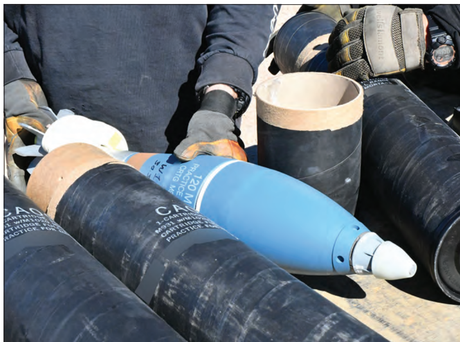
To test the M47 propellant, a wax projectile is used for firing out of the 120mm mortar. If the batch of propellant passes its round of testing, officers will move on to the ignition cartridges and propellant charges. (Photo by Brandon Mejia)
