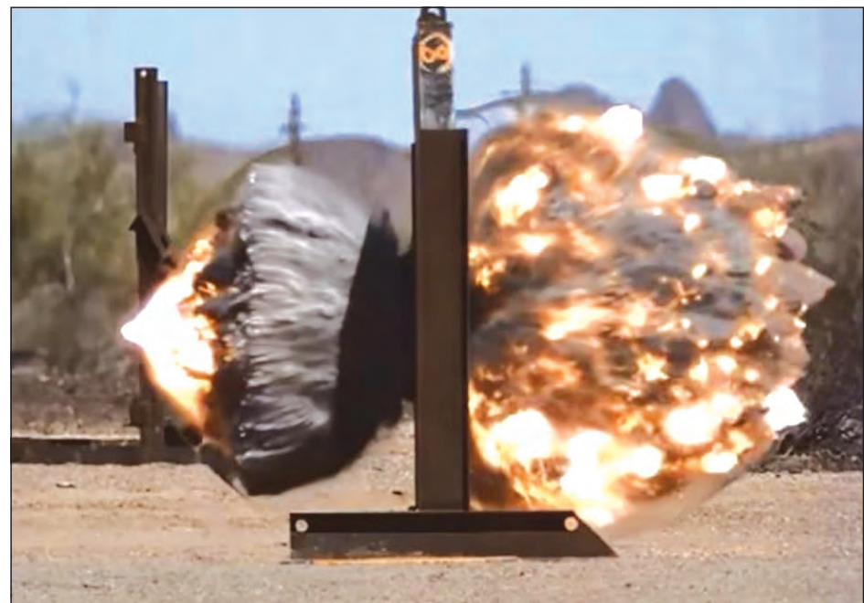
An XM-1147 Advanced Multi-Purpose (AMP) round test shot showing effectiveness against a reinforced concrete wall. (U.S. Army)
