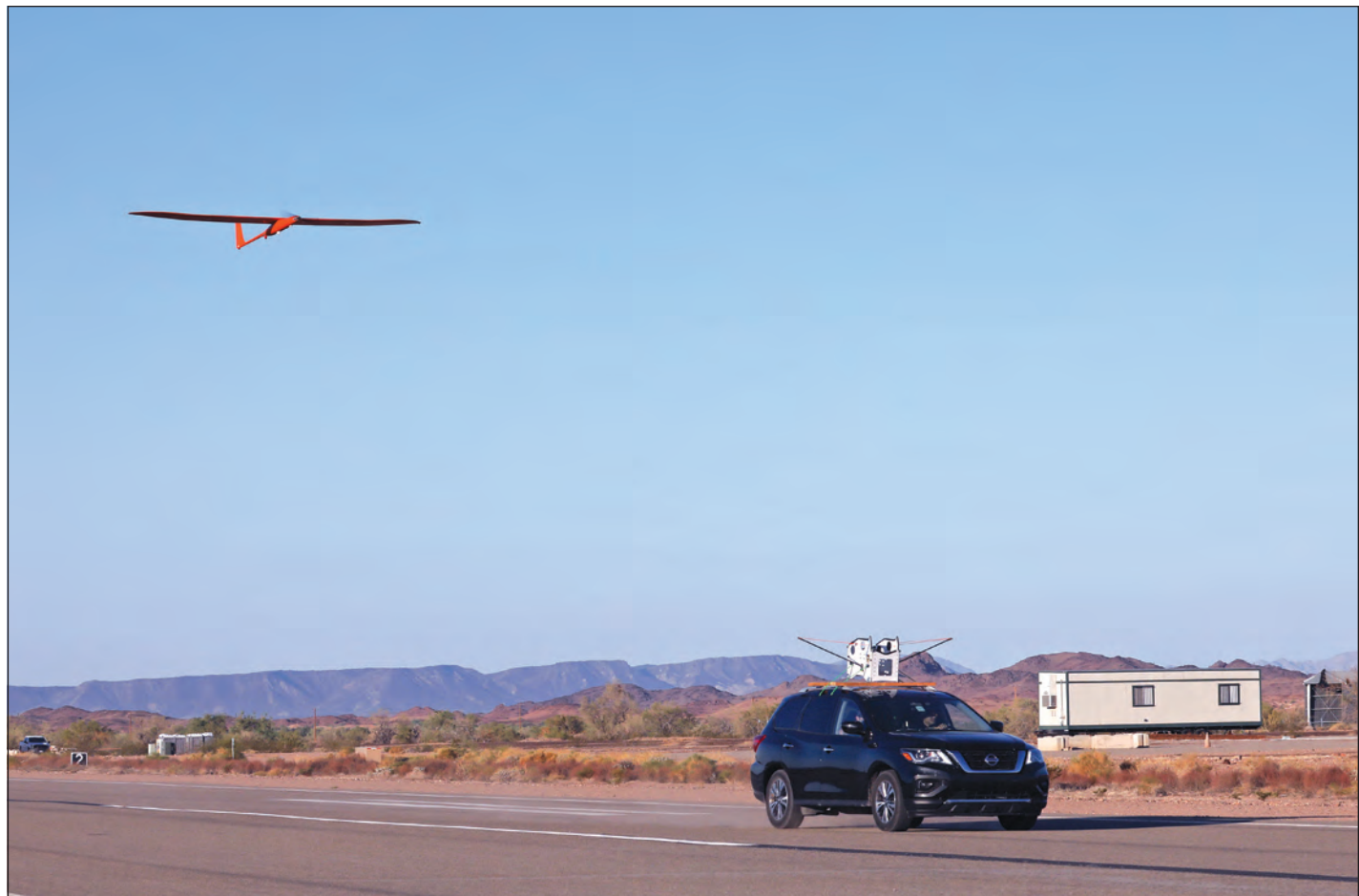
One of the more exciting technologies used was Air Launched Effects drones attached to a helicopter or other vehicle that can be an aviator's eyes in an area of interest. These remarkable and low-cost surveillance UAS can also be launched off of light ground vehicles. An A K-1000 ultra-long endurance is pictured in flight. (Photo by Spc. Cody Rich)
