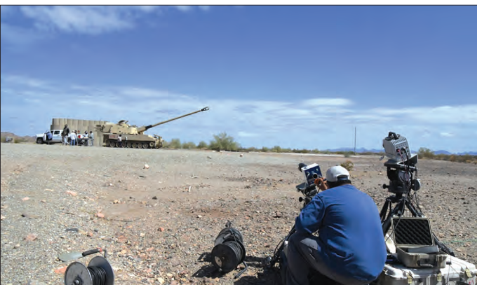
The data collection is critical in developmental testing. High-speed video technician Chris Conner verifies the setting on the camera to ensure it captures video of the projectile as it exits the cannon. (Photo by Ana Henderson)
