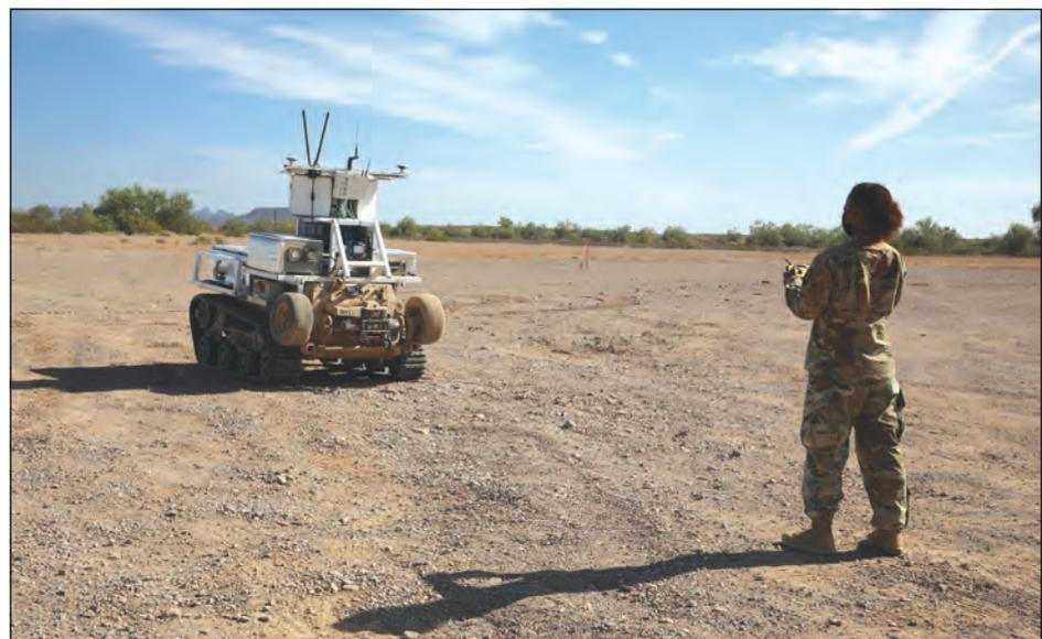
U.S. Army Spc. Destiny Jones, navigates a Robotic Combat Vehicle during Project Convergence at Yuma Proving Ground. The Next Generation Combat Vehicle Cross-Function Team is experimenting with using the vehicle for semi-autonomous resupply, helping Soldiers get the materials they need on the battlefield. (Photo by Spc. Kayla Antsey)
