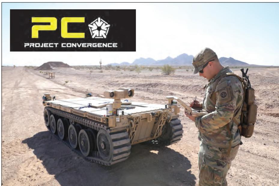
U.S. Army Pfc. Daniel Candales, assigned to the 82nd Airborne Division, uses the tactical robotic controller to control the expeditionary modular autonomous vehicle as a practice exercise in preparation for Project Convergence at Yuma Proving Ground. During Project Convergence 21, Soldiers are experimenting with using the vehicle for semi-autonomous reconnaissance and re-supply. (Photo by Sgt. Marita Schwab)
