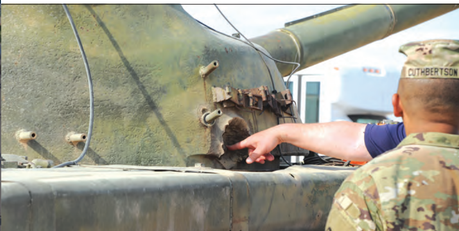
One main battle tank in the test fleet has multiple impacts from previous test fires of predecessor munitions while the vehicle was being autonomously controlled. For this test, rather than detonate the rounds, the XM204’s on-board sensors use a camera reticle to take a photo of the point of deployment.
