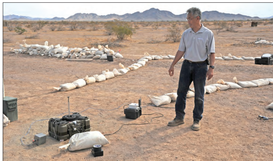
YPG’s test site is highly instrumented and designed specifically for this type of testing. Built in the mid-1990s, the site is intricately networked with fiber optic cable and hard power lines, without which noisy generators that could interfere with the testing. (Photos by Mark Schauer)
