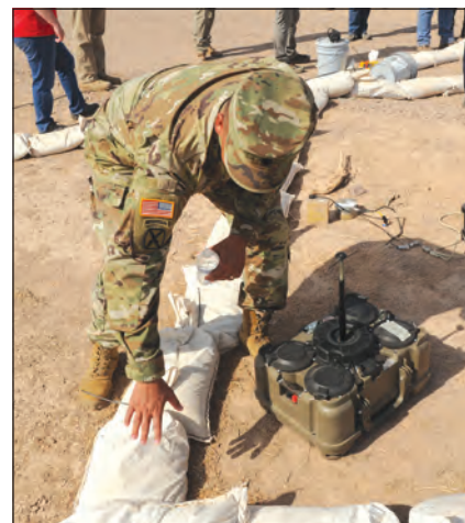
Testing of the XM204 interim wide area top attack munition took place at Yuma Proving Ground. The launcher's large carrying handle came as a result of combat engineer feedback during a Soldier touchpoint. (Photo by Mark Schauer)
