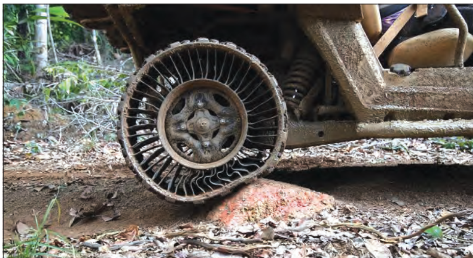
Tropic Regions Test Center recently conducted a test with a military grade Polaris MRZR outfitted with Tweels instead of standard tires. The Tweel, produced by Michelin, is an airless radial tire designed to work like an ordinary pneumatic tire. (Photo courtesy of Tropic Regions Test Center)
