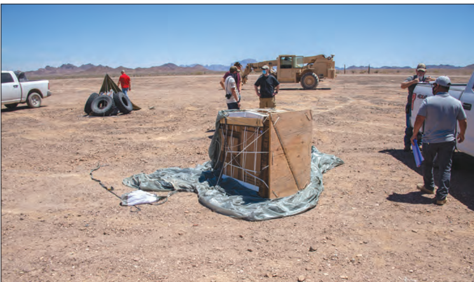
The Autonomous Aerial Insertion and Resupply into Dense Urban Complex Terrain (AAIRDUCT) Joint Capability Technology Demonstration at Yuma Proving Ground, involved the precision delivery of payloads of between 50 pounds and 2,400 pounds to units in urban environments. (Loaned photos)
