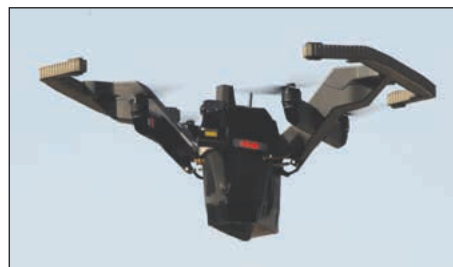
When the vehicle is shifted from ground-based to air-based mode, its ground tracks rotate up to become propeller guards.
