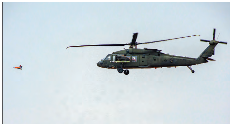
An Air Launched Effects system is launched from a UH-60L Black Hawk as part of capabilities testing during Project Convergence at U.S. Army Yuma Proving Ground. The autonomous weapons system was designed to launch from in-flight aircraft at high tactical altitudes. Project Convergence's capstone event was the Army's largest capabilities demonstration of the year. (Photo by Spc. Javion Sidors)
