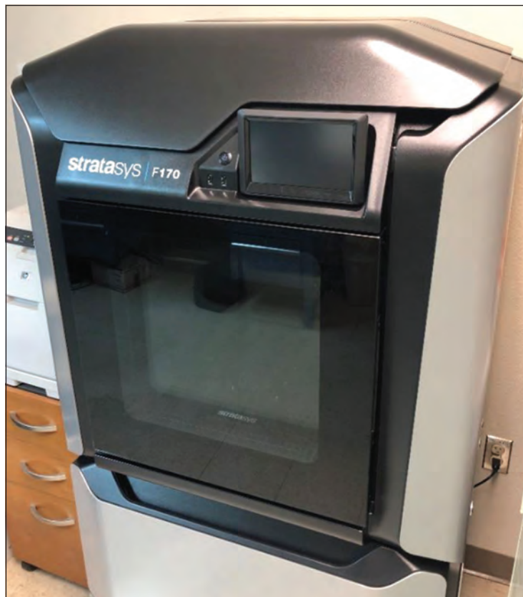
YPG recently purchased a Stratsys F170 printer that can print different materials including a rubberized material (TPU 92A) which opens up the possibilities for printing non-ridged designs. (Photo by EM Lab)
