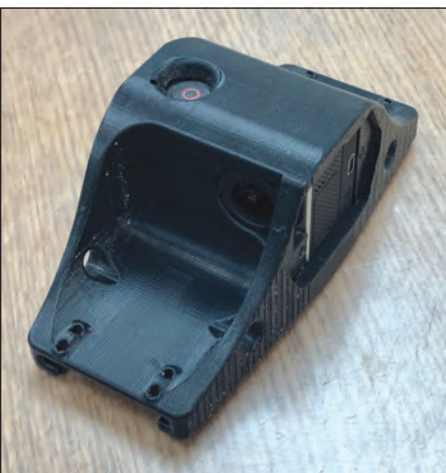
Bob Bieser worked closely with the Airborne Test Force to create an enclosure for a GoPro camera. ABOVE: This image shows the rendering of the design and BELOW: here is the printed product. (Photos by EM Lab)
