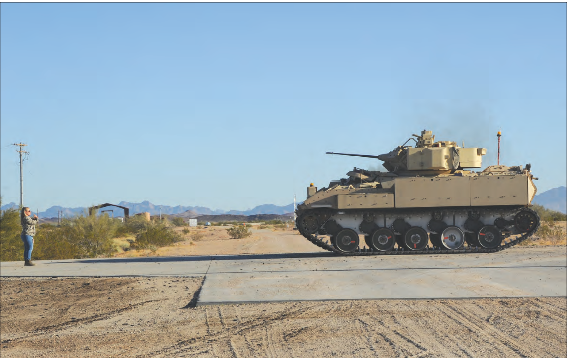
YPG has been testing the Ground Vehicle Systems Centers Advanced Running Gear for potential use on the future NGCV Operationally Manned Fighting Vehicle. The ARG system is using an existing Bradley Fighting Vehicle as a surrogate test platform. (Photos by Mark Schauer)
