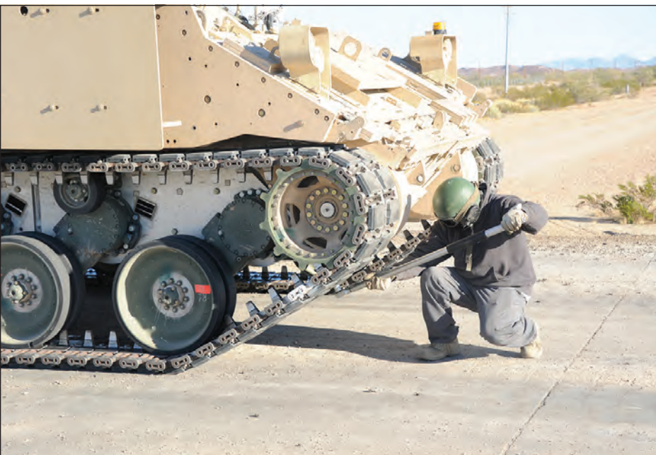
During performance testing, the evaluators collect roughly 100 channels of data, including the displacement and temperature of each road arm as they are put through their paces.
