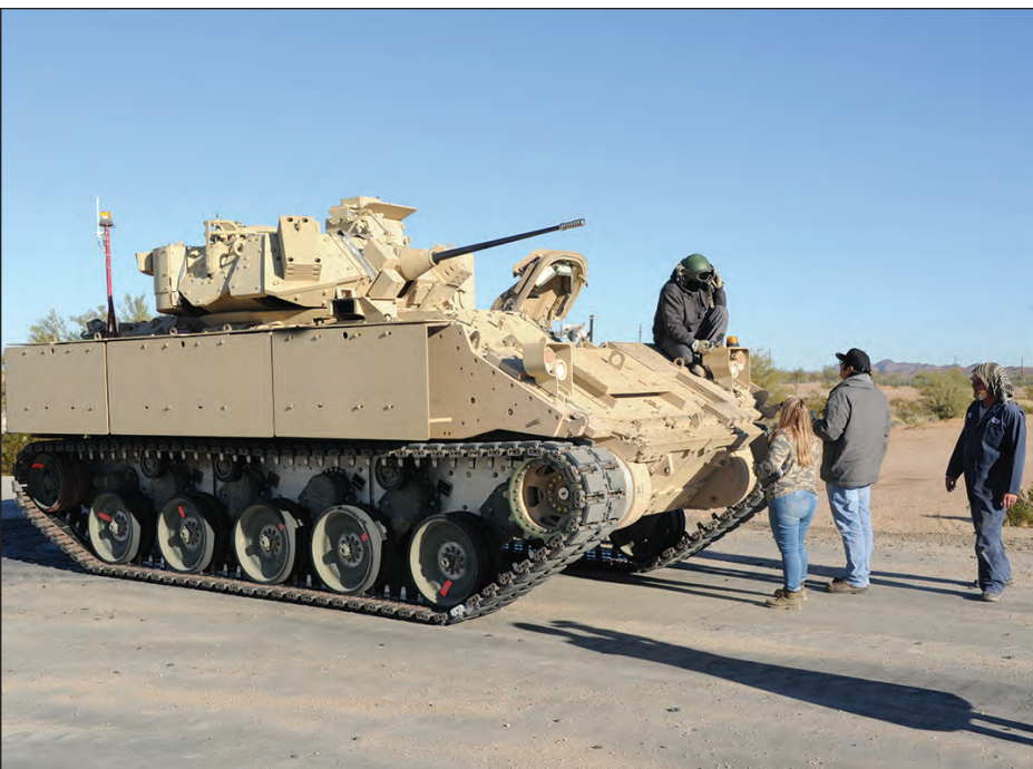
“We’re doing a proof of concept test for the road arms, road wheels, and track tensioner for the vehicle,” said Jade Janis, test officer. “The intent is to improve the ride quality and durability.”
