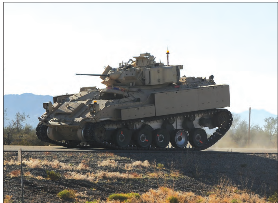
“We’re doing a proof of concept test for the road arms, road wheels, and track tensioner for the vehicle,” said Jade Janis, test officer. “The intent is to improve the ride quality and durability.”
