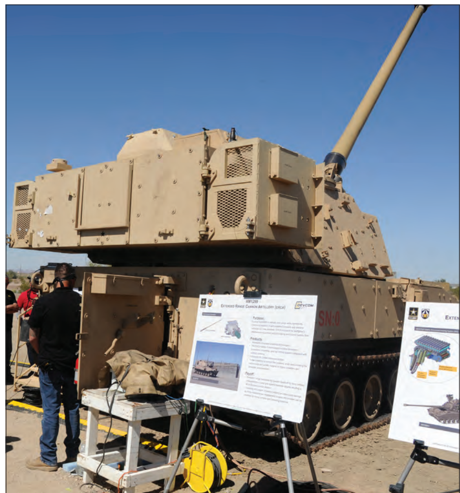
The performance of the XM 1299 self-propelled howitzer, outfitted with a 58 caliber tube on a PIM chassis with loader assist, was the centerpiece of the test.
