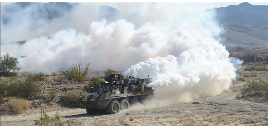
"We ran the vehicle with the smoke generating over a number of different terrain types," said Steve Wilson, test team lead. "We wanted to test the endurance of the system and determine its ability to perform as designed across multiple terrains."
