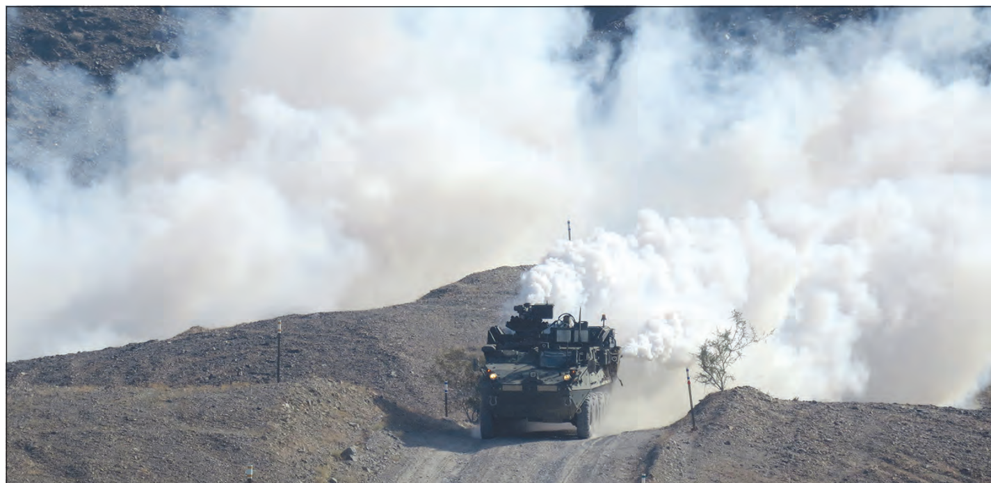
"The fog oil is never burnt: it just becomes atomized," said Michael Shine, test officer. "Then it gets injected out and coalesces into fog. The fog oil used to generate the smoke is purchased in accordance with tight specification and is as harmless as vegetable oil." (Photos by Bob Filinger)
