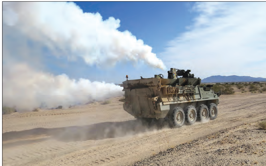
The XM75 Screening Obscuring Module recently tested at Yuma Proving Ground protects Warfighters by obscuring their vehicle from the enemy's vision. (Photo by Bob Flinger)
