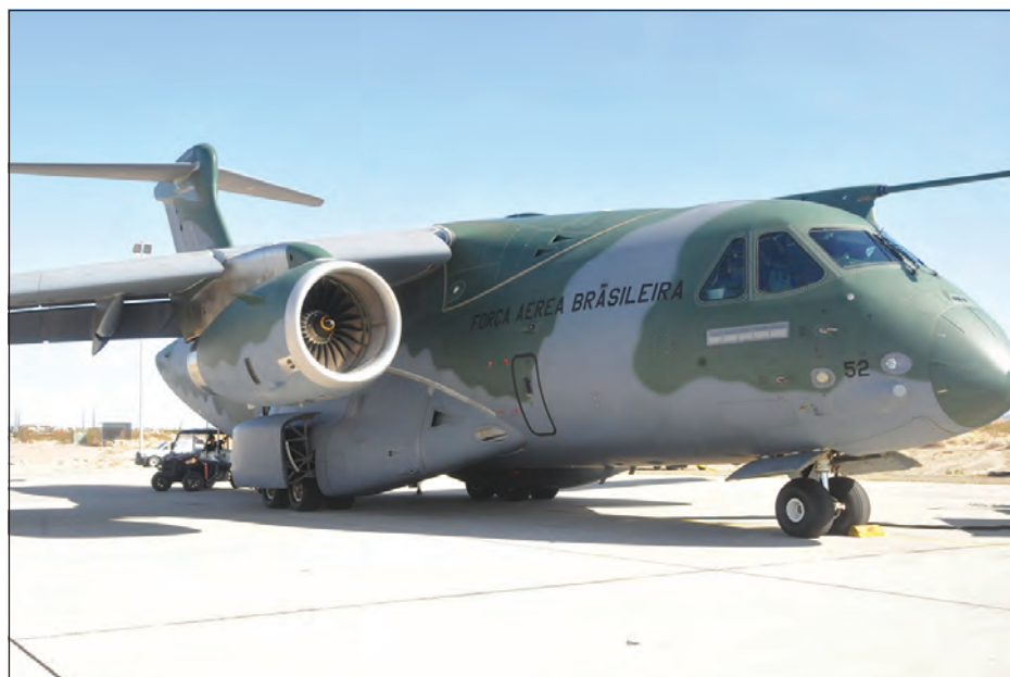
Embraer, a Brazilian aerospace manufacturer, is back at YPG continuing the aircraft certification of the KC-390. The Embraer KC-390 is a twin-engine jet-powered military transport aircraft with multi-functional use. (Photos by Ana Henderson)
