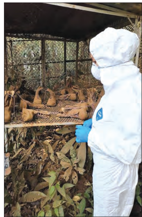
The testers conducted an exposure test where two pairs of each variant of the boot were placed in locked double fence exposure cages set within a triple canopy jungle, where they laid in the ankle-deep leaf and biomass-strewn ground for four months. (Photos by Mark Schauer)
