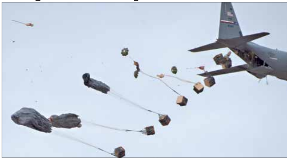
The Extracted High-Low Speed Container Delivery System uses a new G-15 cargo parachute along with an extraction parachute to also have the capability of rapidly dropping bundles at airspeeds of up to 230 knots, keeping them in a tighter pattern and greatly reducing the aircraft's exposure time over a drop zone. (Photos by Mark Schauer)
