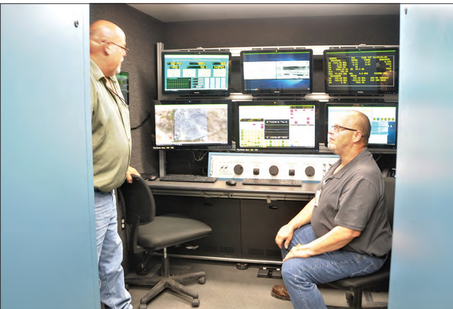
This is glimpse of what the inside of the FPS-16 radar control room. While that radar has an instrumentation truck attached with cables, it can also be used without the truck. It is self-contained and can be operated remotely via a remote console. (Photos by Ana Henderson)
