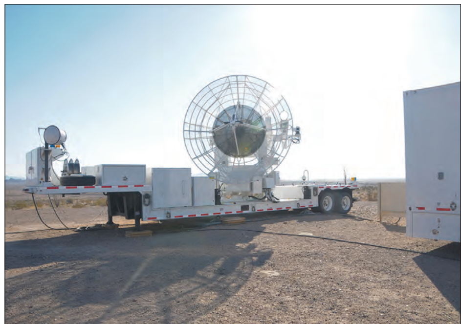
YPG has one radar, the FPS-16 which is part of the RRRP program but is a rebuild and not a commercial off-the-shelf system. The FPS-16 radar is self-contained and can be operated remotely via a remote console.
