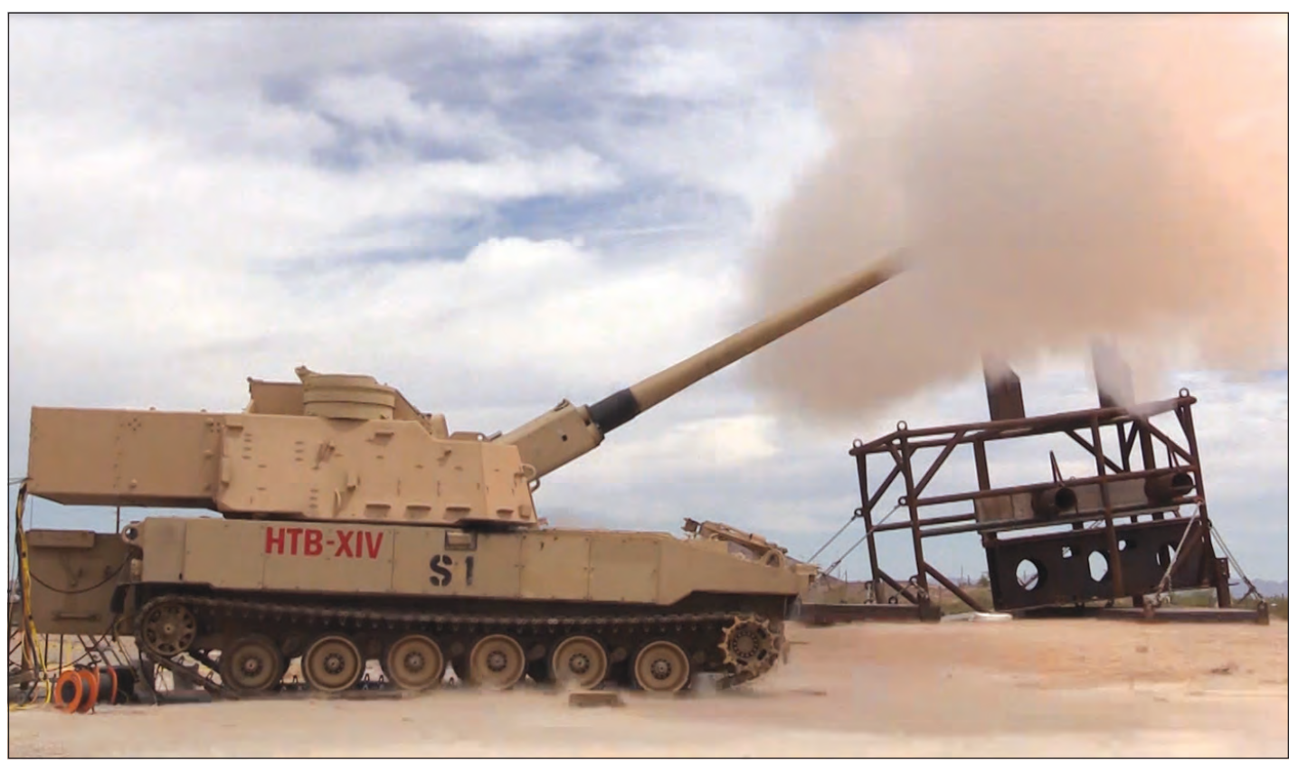
The ERCA program has been testing various components of its system for about four years. The newest component undergoing testing is a five-round limited capacity autoloader. It holds five projectiles and five propellant charges. (YPG loaned photo)
