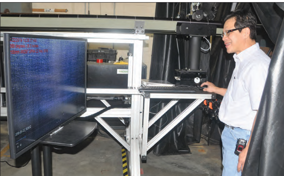
The high-definition video camera system goes into the cannon tube, then using the mouse and computer monitor an inspector can adjust the focus and lighting of the camera to see very fine details.
