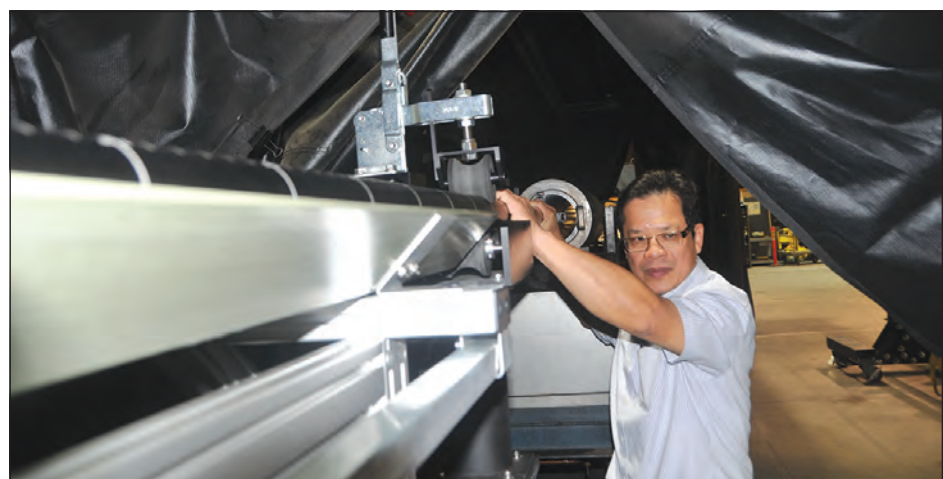
YPG purchased the High-definition Ultraviolet Visual Borescope inspection system which is used for visual borescope inspection and the magnetic particle inspection of the cannon gun barrel. It has the capability to inspection 105, 120 and 155mm cannon tubes.
