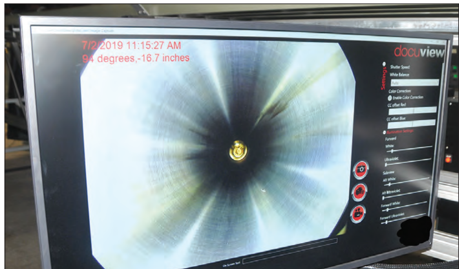
The system software shows the position and location (angle and axis) of the camera (when inside the cannon tube) on the screen, allowing inspectors to pin point exactly where cracks are located. “If we see any type of feature show up on the screen, we are able to see the location” says Le.
