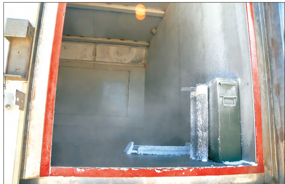
This is the inside of one of the freezing conditioning chamber units. Temperatures range from -60 to +160 degrees Fahrenheit.
