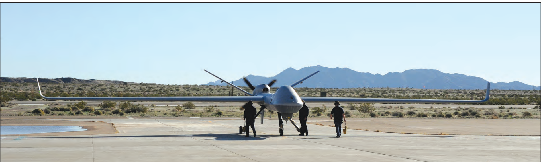
While current ground control stations are bulky, vehicle-mounted cabs that need a prime mover to transport and a support crew to man, the Sky Guardian is controlled by a highly portable laptop computer, cutting the ground crew down to more than three individuals.
