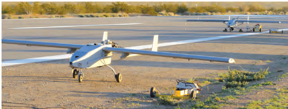
In recent tests at YPG, unmanned aerial vehicles equipped with DARPA's Collaborative Operations in Denied Environment (CODE) system successfully carried out mission objectives, even when communications were offline and GPS was unavailable. The Tigersharks unmanned aircraft employed in the demonstration are surrogate assets for CODE. Each has about one-tenth the speed and performance of the aircraft planned for integration, but shows traceability to larger platforms. (US Army photo)
