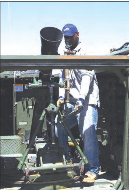
With a mechanized mortar carrier, the scope of evaluation goes far beyond firing. The repeated shock produced by a 120mm mortar's recoil can adversely impact the vehicle's engine mounts and suspension system, requiring YPG testers to take a holistic view of a system. (Photo by Mark Schauer)
