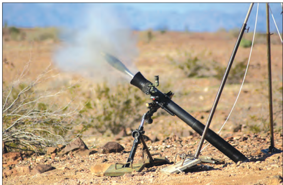
The ballistic tubes used by YPG mortar testers are outfitted with holes to accommodate pressure gauges and other instrumentation. For a conventional mortar, YPG testers gather information like chamber pressure and velocities, and measurements of the range and deflection of the projectile's point of impact. (US Army photo)
