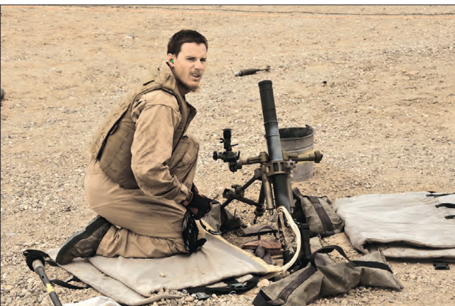
YPG gunners typically do not fire the test projectile by dropping it into the tube as a Soldier in combat would. In the rare instances where a test requires fire that replicates actual use, the gunners, many of whom are uniformed artillery veterans, wear Kevlar vests and helmets and follow other safety precautions. (Photo by Mark Schauer)
