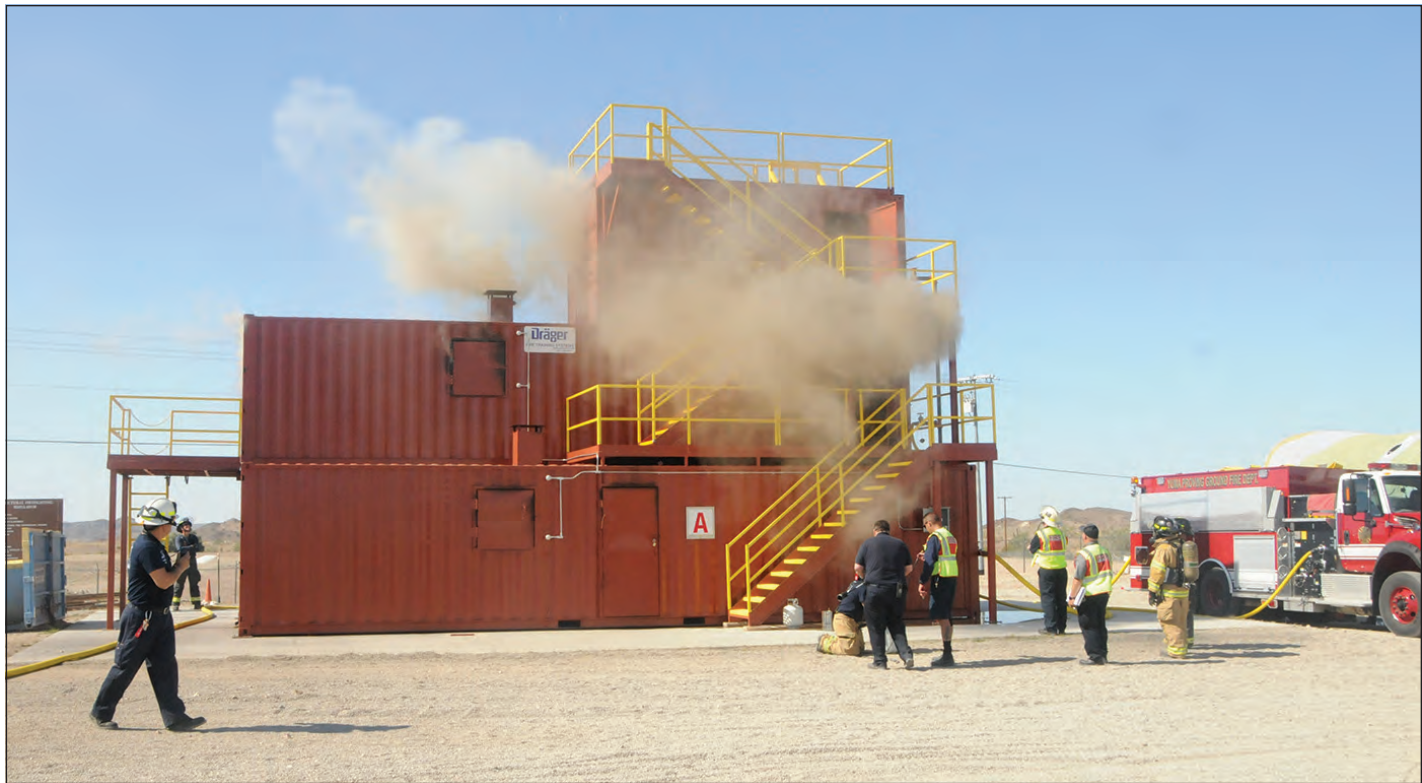
Though the burns were strictly controlled for safety, temperatures inside the fire on the upper floor of the simulation building approached 900 degrees Fahrenheit and visibility was severely impaired by acrid smoke.
