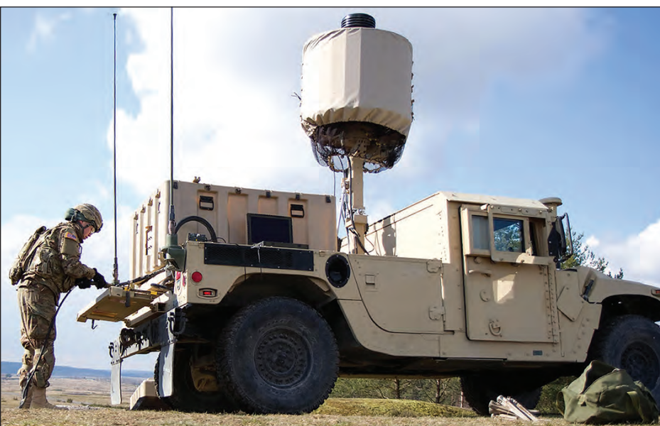
The AN/TPQ-50 counterbattery radar plays a key part in a JPEO-CBRND experiment at Yuma Proving Ground, providing radar data in which the experiment will look for information on CBRN threats. The experiment's aim is to determine whether radar systems like the AN/TPQ-50 and AN/TPQ-53 can detect ordnance filled with chemical or biological weapons or materiel, either in flight or upon detonation. (U.S. Army photo)
