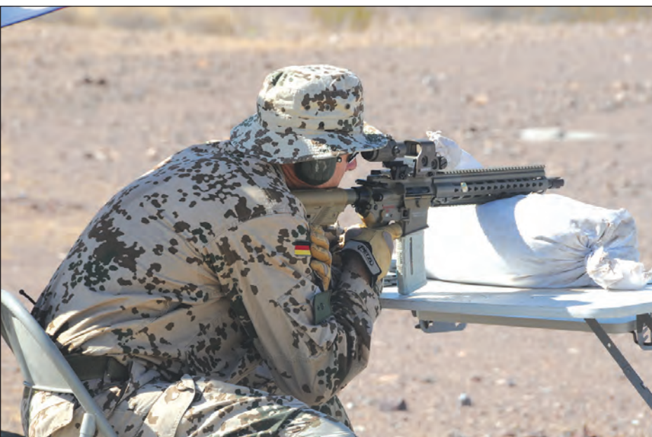
Prior to fielding the new weapon, the testing was conducted to answer a number of questions: How well can the weapon be handled by infantrymen whose hands are slippery with gritty sweat? Will it still function in dust and dirt, even when it isn't cleaned for several days? American Army testers ask similar questions when testing their own equipment. (Photos by Mark Schauer)
