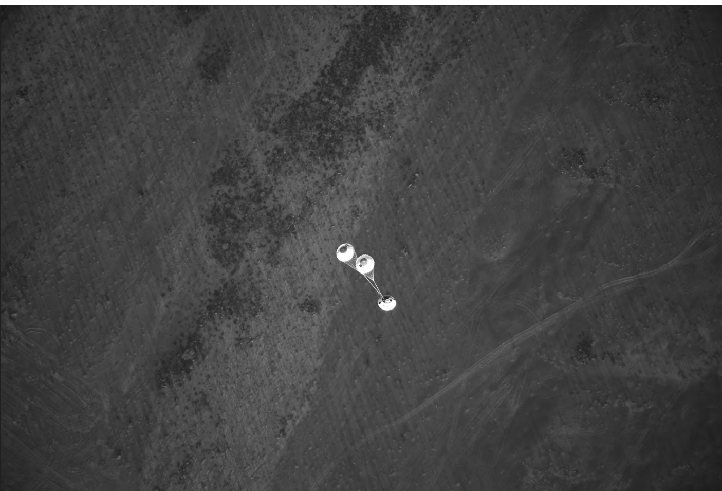
During the test, a mock-up of the Orion spacecraft was dropped from a C-17 aircraft flying at 35,000 feet. The evaluation was of a simulated scenario in which one of the three main parachutes failed to open after the deployment of several drogue parachutes that help slow and stabilize the spacecraft. (US Army photo)
