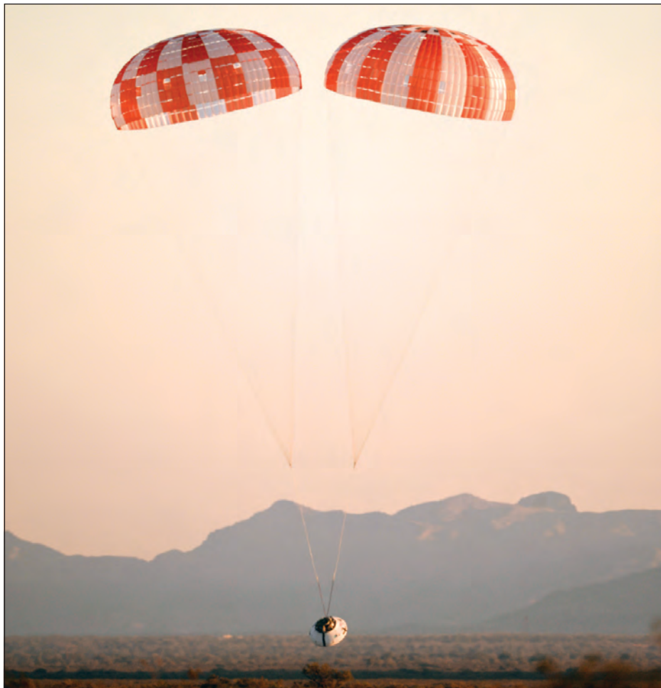
NASA successfully conducted the fifth in a series of eight tests to qualify the parachute system for crewed Orion space capsule missions at U.S. Army Yuma Proving Ground in late December. Orion's parachutes help slow the capsule from about 300 mph to less than 20 mph in under 10 minutes and are critical to the safe return of the spacecraft and its future crews after deep-space missions. (US Army photo)
