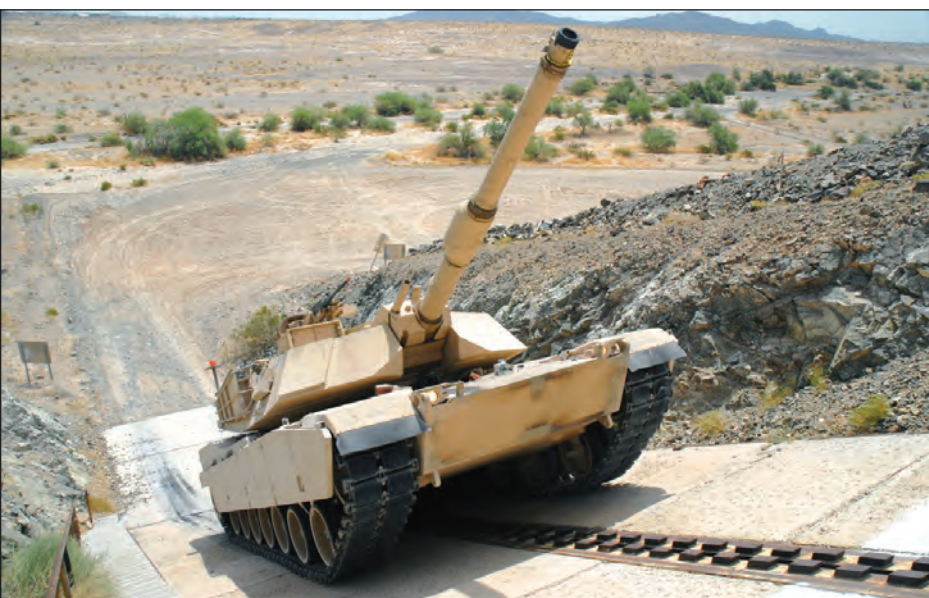
Yuma Proving Ground's Combat Automotive Systems Directorate puts military vehicles through a grueling reliability and performance regimen amid pristine desert terrain. When not racing across scores of miles of hot, treacherous desert road courses, vehicles like this M1 Abrams tank are put through other stresses, such as climbing this awing 60% grade. In comparison, the steepest grade on an American interstate highway is 6%. (Photos by Mark Schauer)
