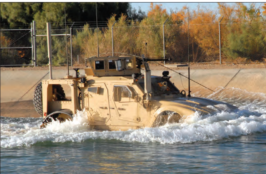
When testing a combat vehicle, YPG test officers plan for dangers unimaginable to a civilian motorist: If the vehicle's hull is rocked by a roadside bomb, can five Soldiers in full protective gear escape with weapons at the ready before the vehicle is engulfed in flames? Will the engine stall halfway up a rocky 40% grade after driving through a five-foot deep stream? Here, YPG drivers power through a fording basin in the all-terrain variant of the Mine Resistant Ambush Protected Vehicle. (Photo by Mark Schauer)
