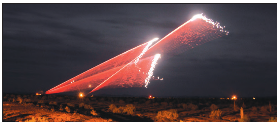
In the earliest days of the insurgency in Iraq, American forces came under frequent attacks that utilized the humble, easily transported mortar. To defend against this threat, the Army assembled the Counter Rocket Artillery Mortar system consisting of the Lightweight Counter Mortar Radar and the AN/MPQ-64 Sentinel radar to detect incoming rounds, and the Land-based Phalanx Weapon System that spits out bursts of fire at hostile projectiles. Thanks to rapid testing at YPG in the early days of the Iraq War, the system was deployed to Iraq in 2005, dramatically reducing mortar and other indirect fire attacks. (Photo by Kurt Harrison)
