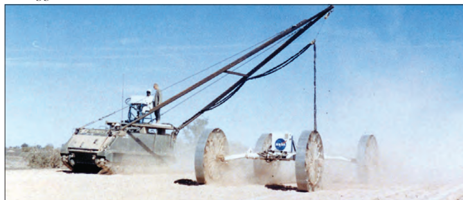
The mobility test article (MTA), a precursor to the lunar rover, came to YPG for engineer design evaluations in 1966. YPG has supported NASA testing since the earliest days of the American space program, and continues to in the present day. (US Army photo)
