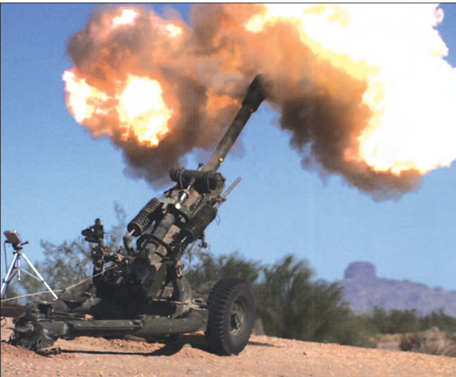
The M119 105 mm howitzer is the lightest, most technologically-advanced indirect fire weapon system in the American arsenal. The 4,500-pound howitzer can be transported by Humvee, 2.5 ton truck, helicopter, or cargo plane. In particularly inhospitable terrain, the howitzer can even be delivered by a single parachute system with the Humvee and 105mm ammunition. (US Army photo)
