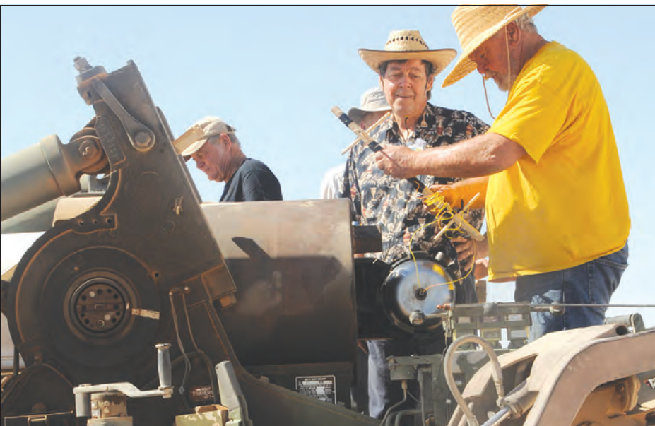
Green Launch employee Ray Tinker prepares the "Christmas tree," the team's term for an ignition assembly with squibs. The testers have already reached velocities similar to that of the HARP vertical shot that set the world record in 1966, and want to achieve even faster velocities before converting to vertical test fires of their system.
