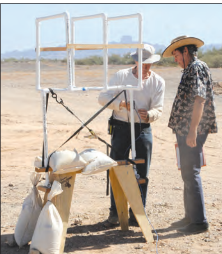
Eric Robinson (left) and Dr. John Hunter of Green Launch inspect a velocity trap prior to a test shot at YPG. The early phase of testing in progress consists of horizontally launching a high density plastic slug through the trap and into a catch box. (Photos by Mark Schauer)
