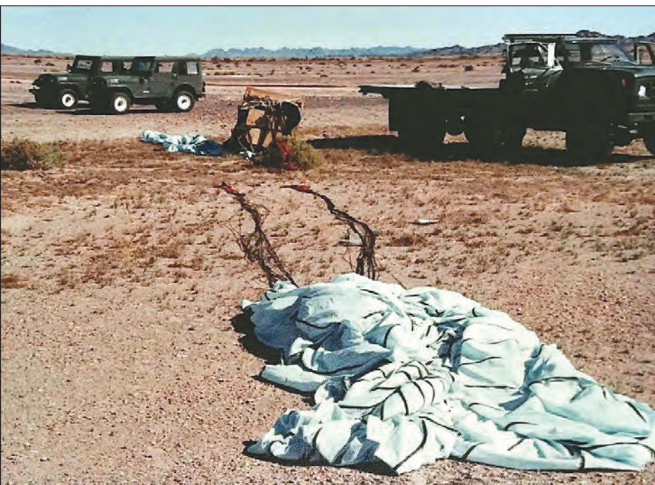
These cargo loads were dropped under a canopy made of a cotton/polyester blend used in bed sheets. Follow-on studies tested canopies made from more-traditional nylon taffeta. (US Army photo)
