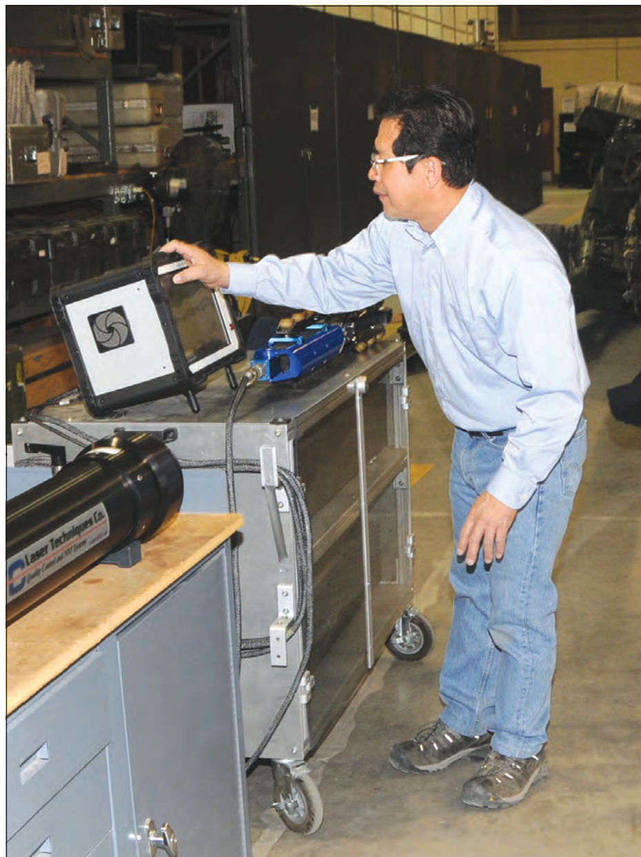
Mechanical engineer David Le prepares to inspect a M777 gun tube using YPG's latest miniaturized, portable laser bore mapper. The quick and reliable range of capabilities in this lightweight package has a dramatic real-life impact on the speed of test and the readiness of equipment that the Warfighter needs. (Photo by Mark Schauer)
