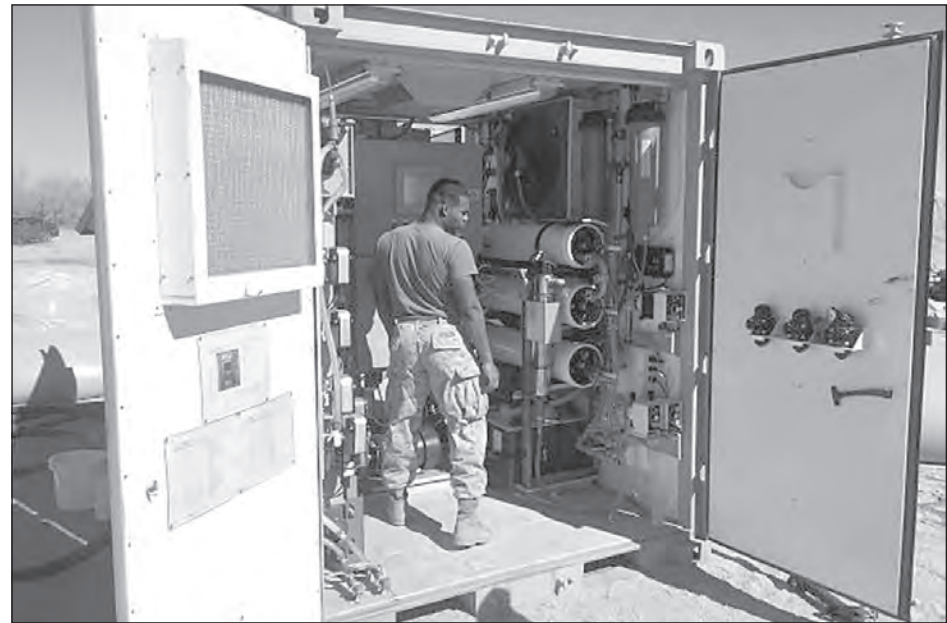
As part of a field exercise at U.S. Army Yuma Proving Ground, members of Marine Aviation Weapons and Tactics Squadron One tested the Shower Water Reuse System (SWRS), part of the Army's "Force Provider" shelter system, over a five-week period. The SWRS captures and reuses 75 percent of gray water, reducing the number of risky resupply convoys necessary to forward operating bases. (Photo by Ryan Eckert)
